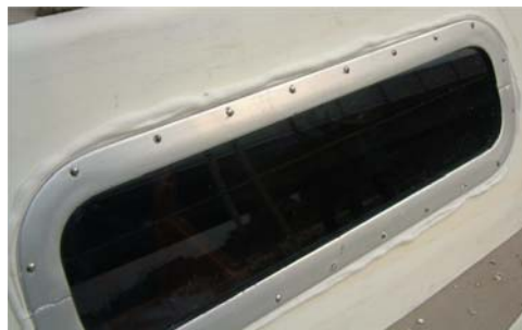
Figure 13: Main Cabin Window Inserted
