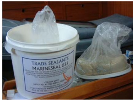
Figure 12: Window 2 Part Putty Sealant
