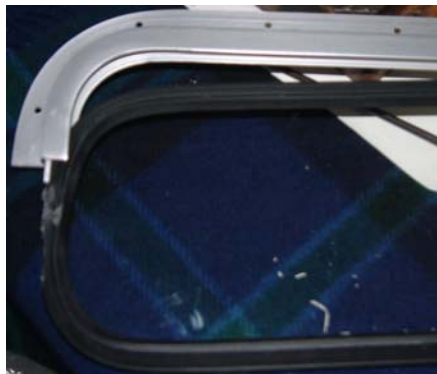
Figure 8: Inserting Glass & Rubber Seal into Frame
