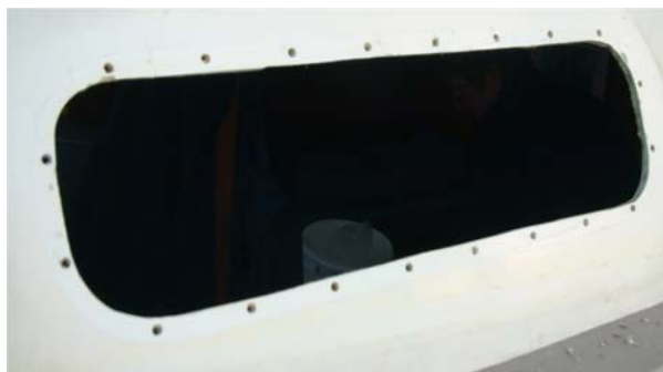
Figure 11: Main Cabin Window: Cut-out, Outside View
